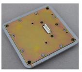
Matrix keypads have locking header P/N 640456-8 Mating connector P/N is 640440-8
