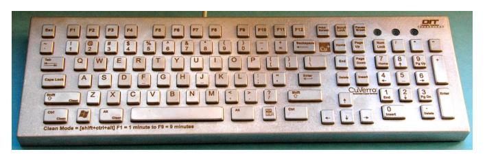
We now have a complete data entry package manufactured with EPA registered CuVerro® bactericidal copper alloy. The keyboard has the feel of a standard computer keyboard and can be cleaned without disconnecting by activating the "clean mode".
